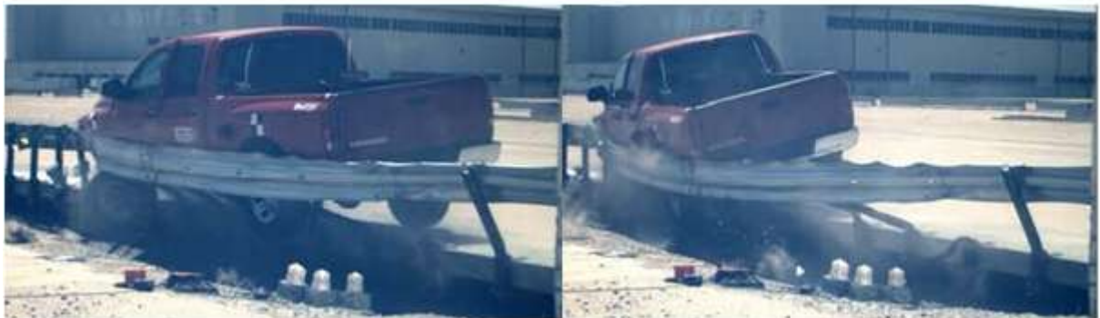
The MGS Bridge Rail Performed Quite Well in High Speed Redirection Crash Tests.
